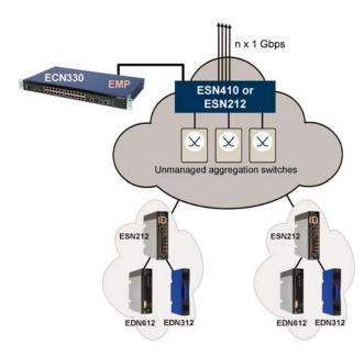
The flexible topology support is particularly powerful for VDSL2 deployment in scenarios where telecom operators already have access aggregation switches in place, with non-Ericsson equipment.
